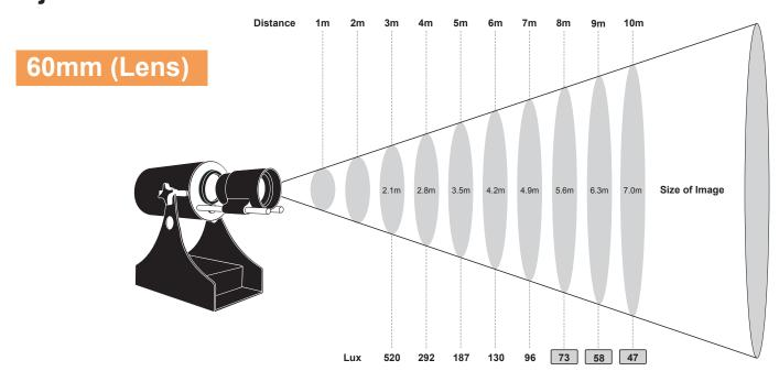
Ratio for Distance 1,4:1 (Image Size - 60mm Lens) The Object Diameter is 42mm
