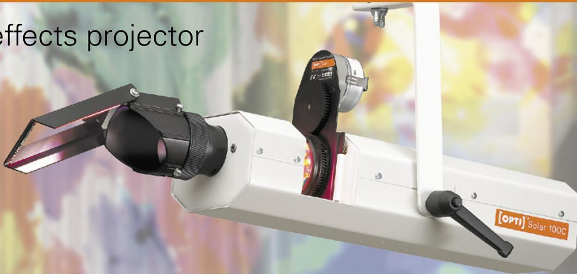
The OPTI Solar 100C is lightweight, compact and simple to use with optical image quality and reliability synonymous with the OPTI name. The OPTI Solar 100C is ideal for close proximity projection, low ambient light conditions and dynamic point of sale or display applications. The OPTI Solar 100C is fitted with a fan cooled quartz halogen 100 watt 12 volt M28 lamp with an average life of 2,000 hours. An 85mm focussing lens is supplied as standard.
