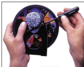
6 inch wheel being fitted to a Solar Wheel Rotator using a small cross head screw driver.
