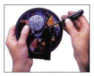
6 inch wheel being fitted to a Solar Wheel Rotator using a small cross head screw driver.
